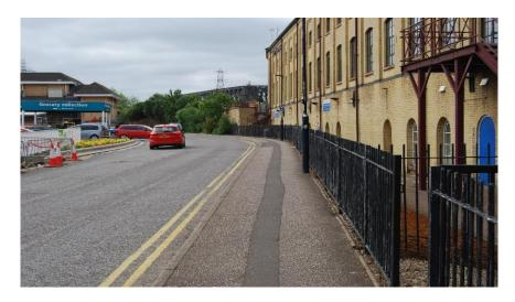
The path along the river is adequate although vegetation is encroaching along the NVR wildlife centre. Immediately after the section recently upgraded the path narrows significantly due to encroaching grass. If this were scraped back at least 0.5 metres of path could be reclaimed.
