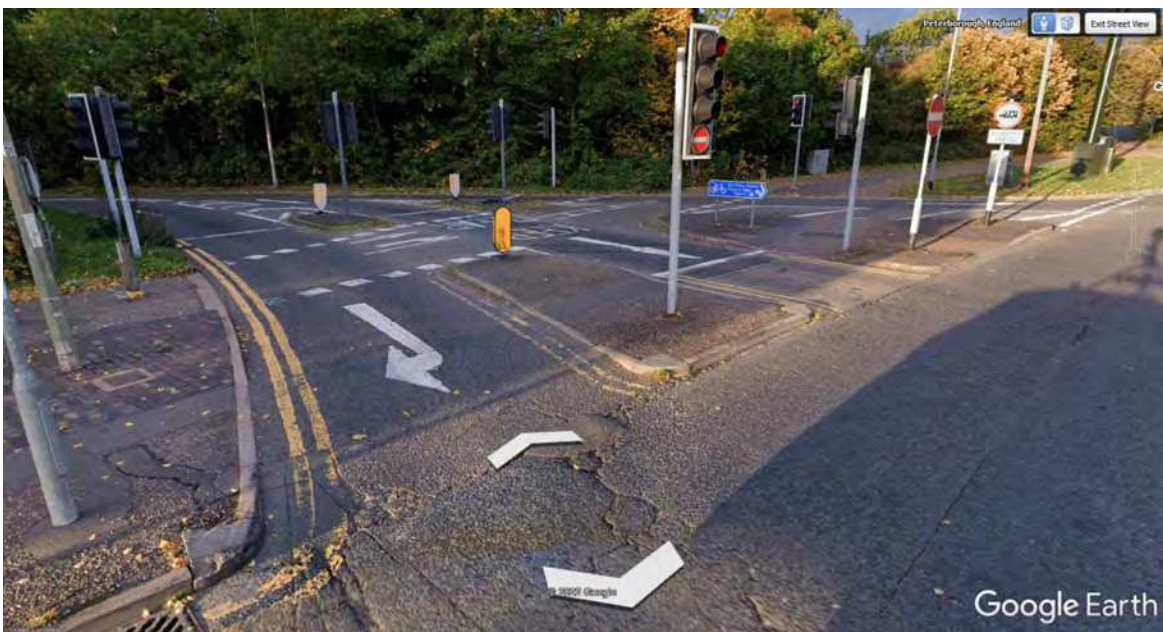
Figure 2.9: Alternate View of Northbound Approach to Junction 7, Showing Poor Cycle Provision Crossing Traffic Lanes (Google, 2022).
