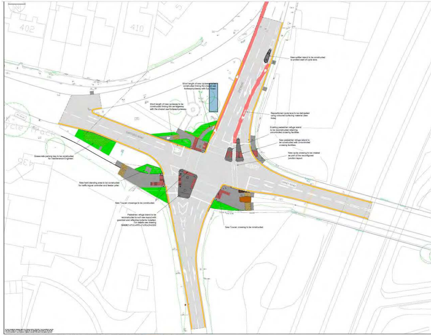
Figure 2.16: General Arrangement of the Junction 7 Scheme
