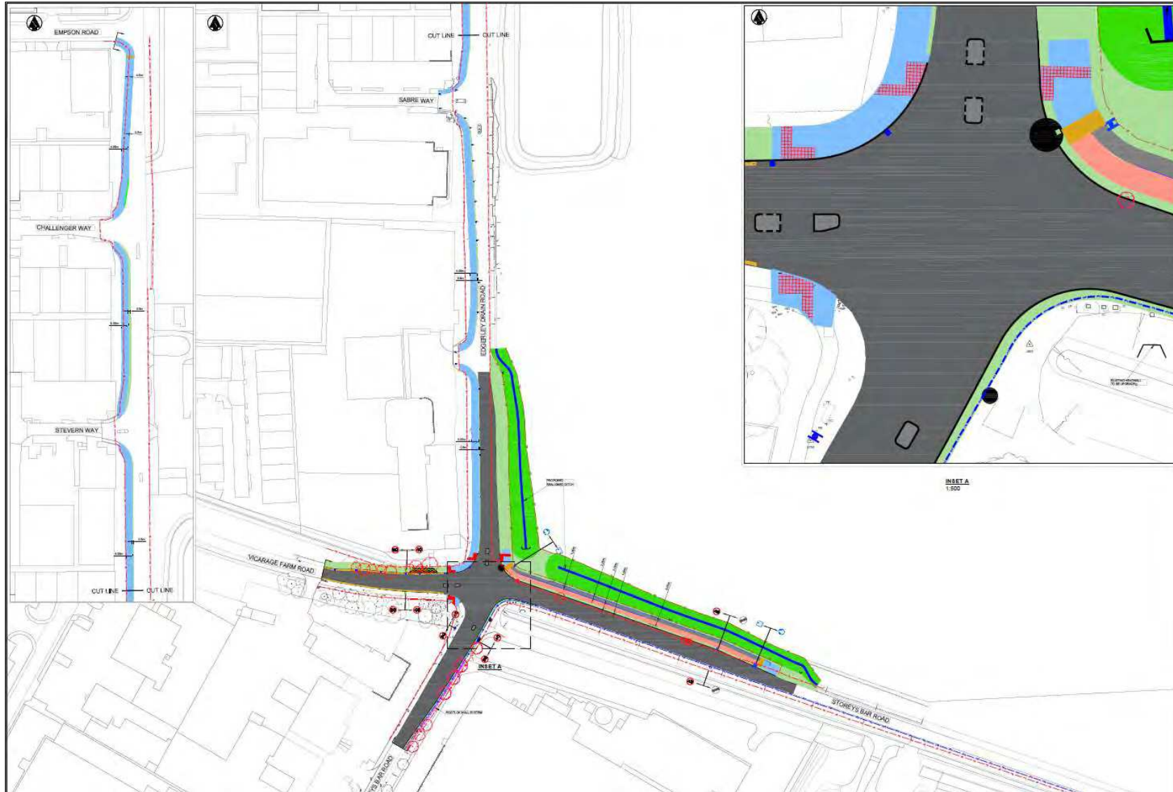
Figure 2.15: General Arrangement of the Edgerley Drain Road / Storey's Bar Road / Vicarage Farm Road Scheme
