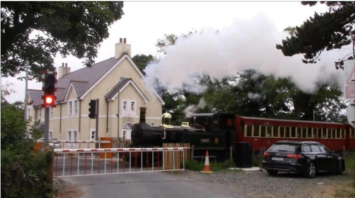
Figure 20 – Simplified Light Rail Barrier Crossing on Isle of Man Steam Railway (Source: YouTube/Perryd Pelle)
