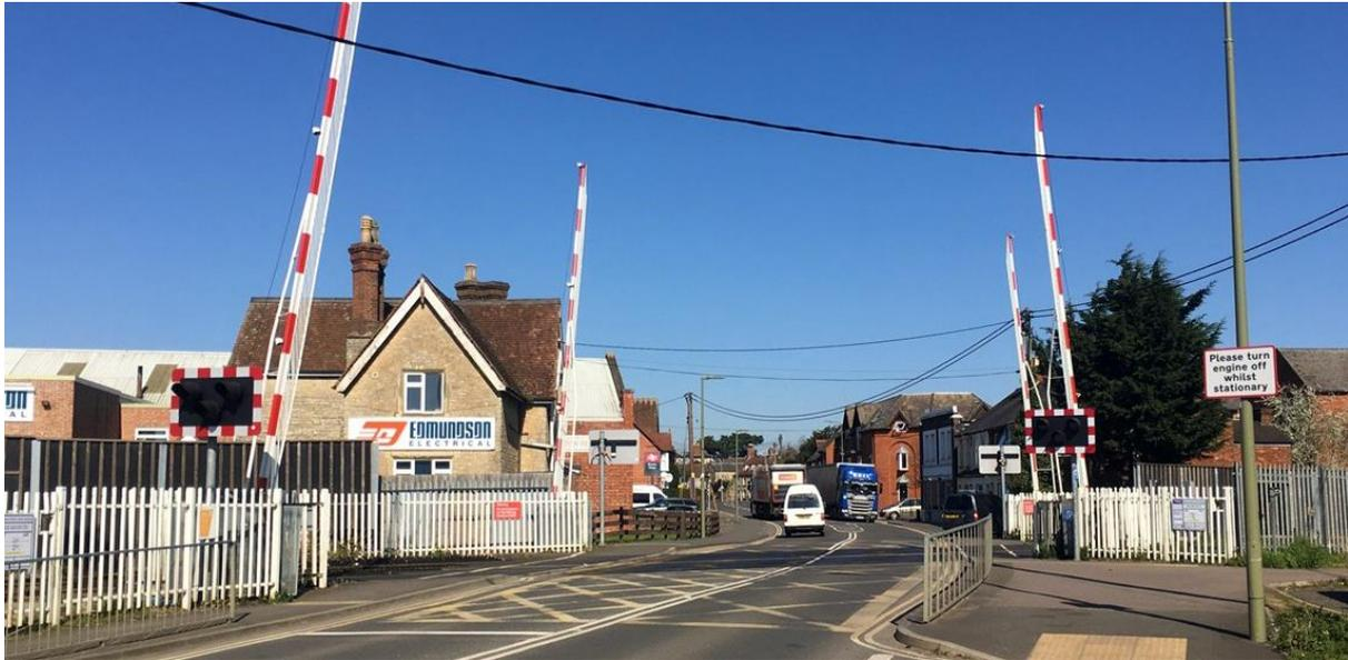
Figure 27 – Typical Full Barrier Heavy Rail Level Crossing (Source: NR Media Centre)
