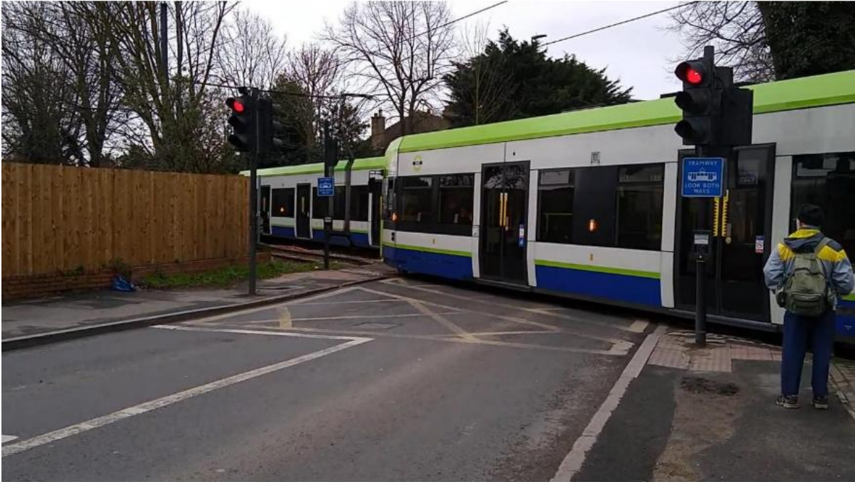
Figure 19 – Standard Tramway Traffic Light Road Junction Crossing (Source: YouTube/MrCrompton 33012)
