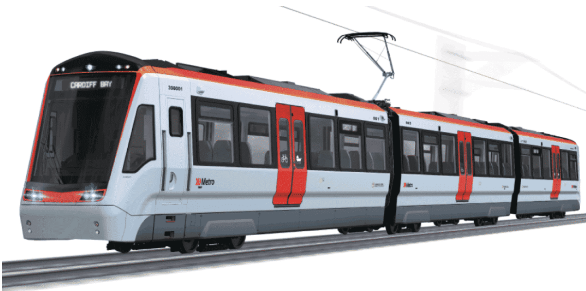
Figure 4 – Class 398 Citylink High Floor Tram Train Under Construction for Core Valley Lines (Source: Transport for Wales)
