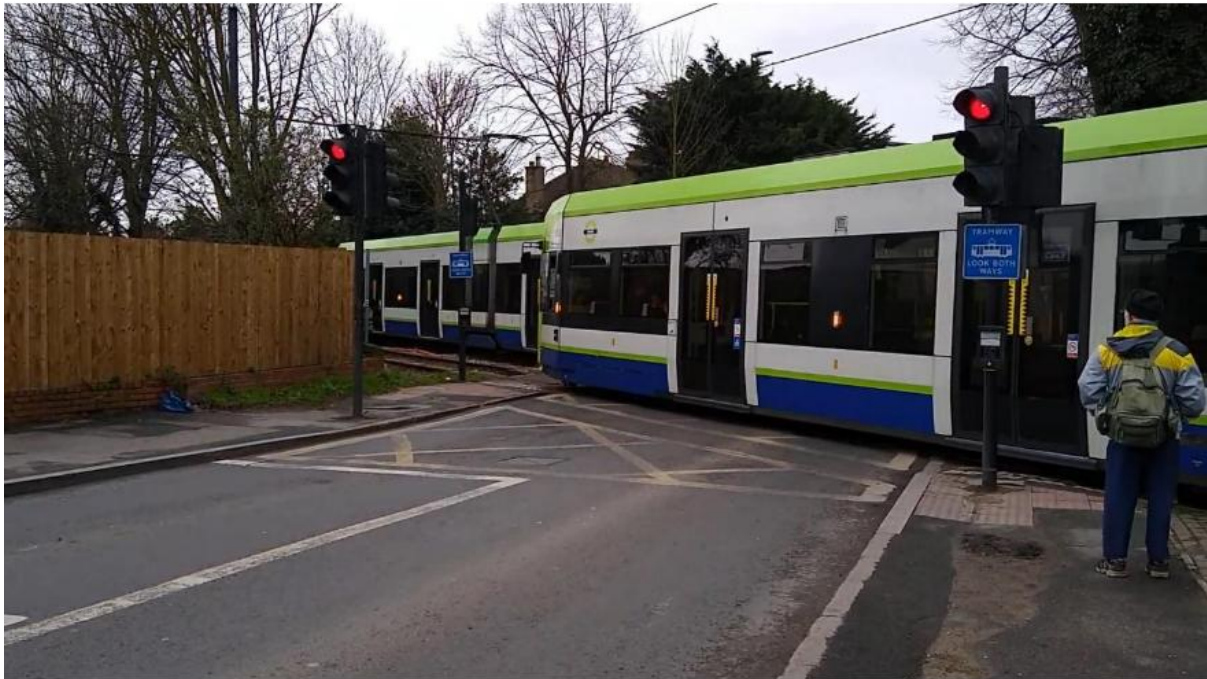
Figure 19 – Standard Tramway Traffic Light Road Junction Crossing (Source: YouTube/MrCrompton 33012)
