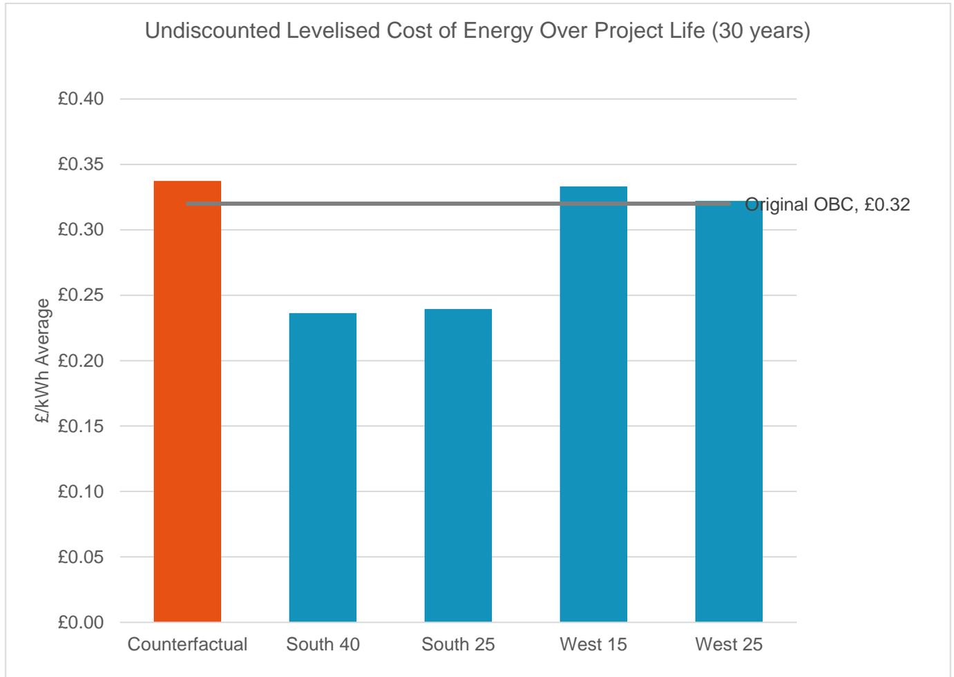
The graph shows that against the counterfactual, the grid connection/reinforcement option, there are technical options for the local grid that significantly outperform the do minimum/counterfactual option. The local grid option with solar PV array southern orientation and 40degree incline is the best performing option based on the analysis to date.
